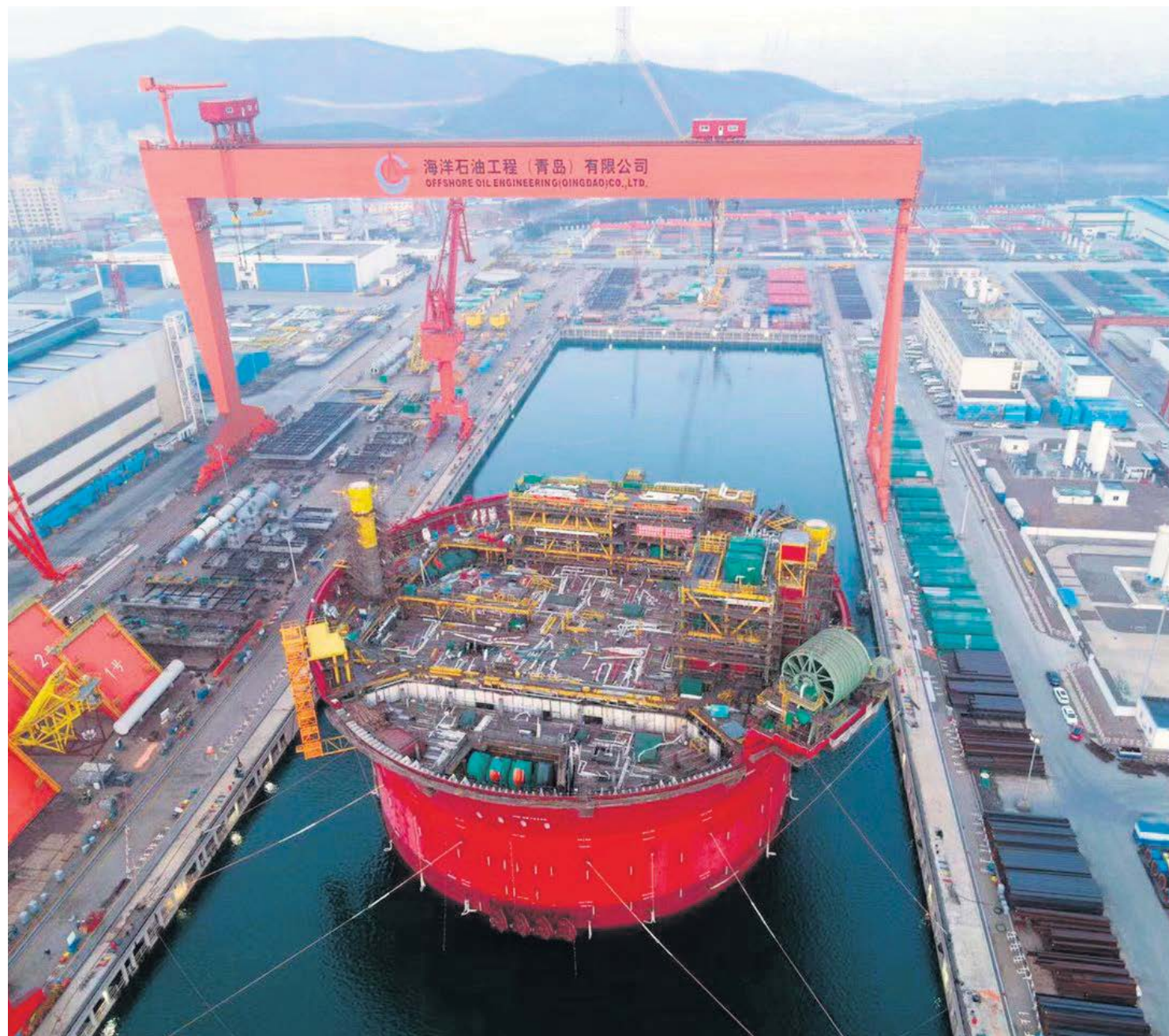
Cylindrical vessel: The Liuhua 11-1 redevelopment is using a similar cylindrical FPSO concept to the one in this image
